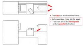
Fig. 1 Bed arrangement on a conventional lathe
